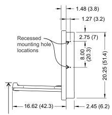
Mounting at maximum height results in this dimension being 34" (86.5), recessed & surface.
