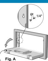
Cradle and recessed panel remain taped together during installation.
